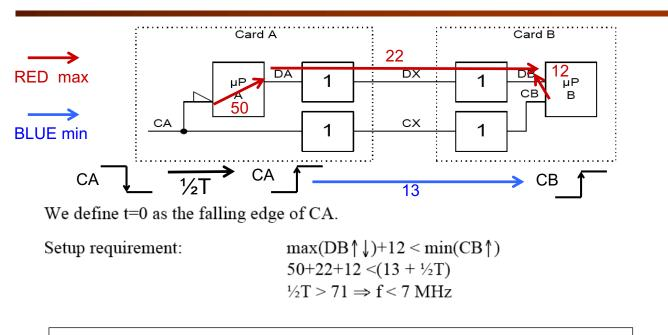
Setup time requirement is governed by the slowest data signal path relative to fastest clock path
