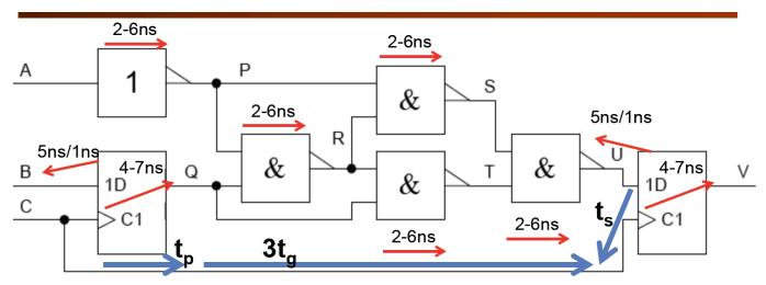
The longest path from C to U passes through the flipflop and then through three gates: this gives a maximum propagation delay of 25 ns. This happens when  $A=0 \Rightarrow P=1 \Rightarrow R=!Q \Rightarrow T=1 \Rightarrow U=!S=R=!Q$ . We therefore use  $3t_g$  in the setup inequality below.
