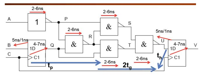
The shortest path from C to U passes through the flipflop and then through two gates: this gives a minimum propagation delay of 8 ns. This happens when  $A=1\Rightarrow P=0\Rightarrow R=S=1\Rightarrow U=!T=Q$ . We therefore use  $2t_g$  in the hold inequality below.
